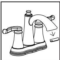
Remove the aerator from the end of the faucet by carefully unscrewing it. Let hot and cold water run through both water lines for at least one minute before replacing the aerator. This will help to clear any debris in the line, which could otherwise clog the system.
